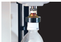
Compression test of plastic bottle
