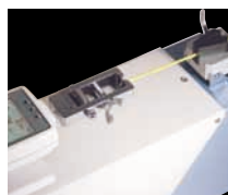
Pull test of a wire harness terminal by LH-500N
