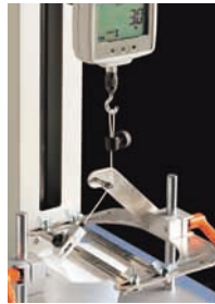
Peeling test of food contain cup
